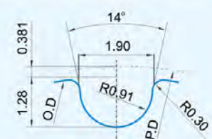
3M轮齿形图 3M Pulley tooth profile figure
