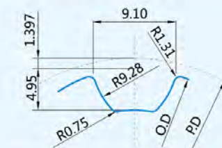
S14M 轮齿形图 S14M Pulley tooth profile figure
