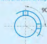
变更止动螺丝角度用KC90表示 Kc90 shows alteration of stop screw angle.
