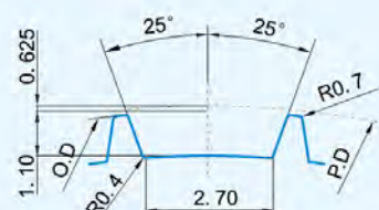
AT5 轮齿形图 AT5 Pulley tooth profile figure
