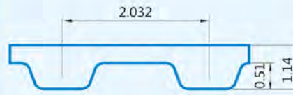
MXL型同步带齿形图 Model MXL synchronous belt tooth figure
