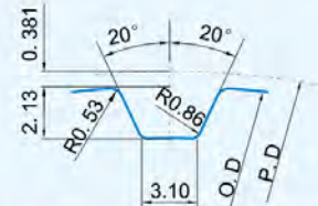
L 轮齿形图 L Pulley tooth profile figure
