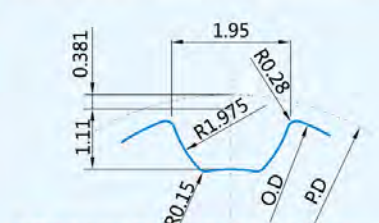
S3M 轮齿形图 S3M Pulley tooth profile figure
