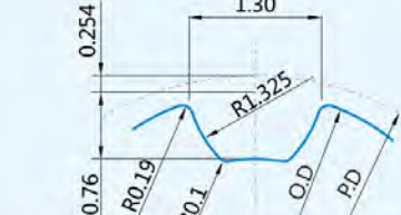
S2M轮齿形图 S2M Pulley tooth profile figure
