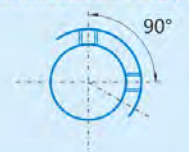
变更止动螺丝角度用KC90表示 Kc90 shows alteration of stop screw angle.
