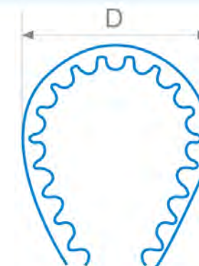
图2 同步带的最小弯曲直径 Figure 2 The miniumum Crimp diameter of timing belt
