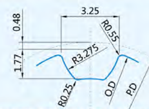
S5M 轮齿形图 S5M Pulley tooth profile figure
