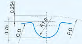
G2M轮齿形图 G2M Pulley tooth profile figure
