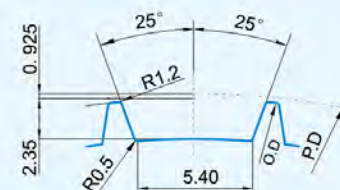
AT10 轮齿形图 AT10 Pulley tooth profile figure
