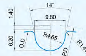
14M轮齿形图 14M Pulley tooth profile figure
