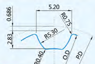
S8M 轮齿形图 S8M Pulley tooth profile figure
