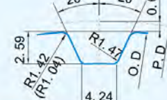
H 轮齿形图 H Pulley tooth profile figure
